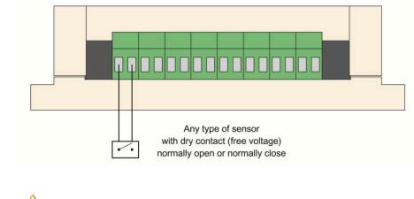
A Only voltage free connection must be applied for contact inputs.
